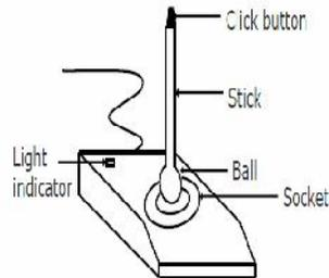
Commonly used for video games, flight simulators, training simulators, and for controlling industrial robots
